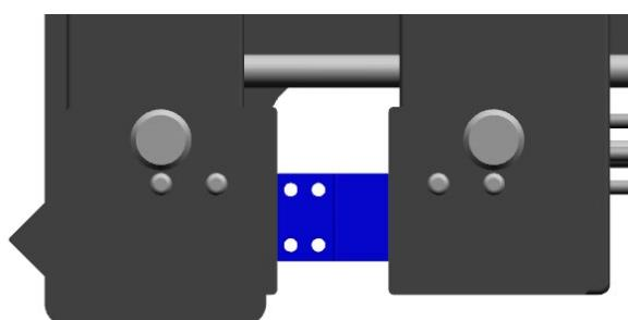
The new variable fixation unit 398054 now includes a tailstock function, a prism holder and a vice with smooth jaws. Part-specific special jaws are available on request. The clamping force can be adjusted very finely and with repeat accuracy via micro springs. 60° tailstock centre pair available as accessory 398060 and can be exchanged for hollow centres.
